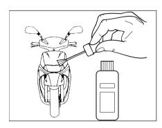
Minor paint damage should be immediately repaired.
