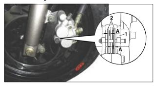
Checking the brake linings
