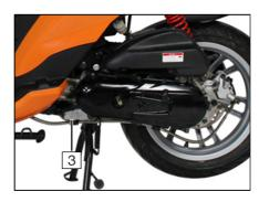
The engine number (3) is located on the left-hand side.
