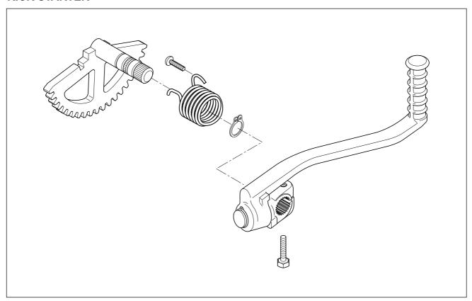
Apply SUPER GREASE "A" lightly on the kick starter shaft rolling surface and install it on the crankcase cover.
