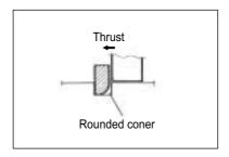
• Install the bearing 4 with the special tool.
