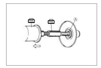
• Remove the circlip <sup>®</sup>.
