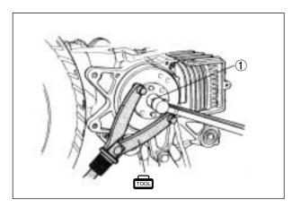
Remove the magneto rotor with the special tool.
