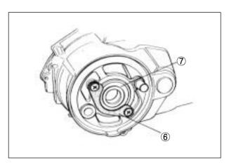
• Remove the bearing ⑦ with the special tool.
