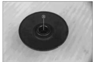
• Remove the bearing © with the special tool.
