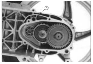
● Apply **BOND** "1215" at the hatched area shown in the illustration and install the gear box cover ① on the crankcase.
