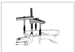
• Remove the bearings, oil seals and bushings.
