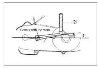
Tighten the kick starter lever bolt to the specified torque.
