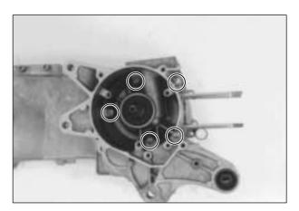
• Install the new oil seal ① to the crankcase with the special tool.
