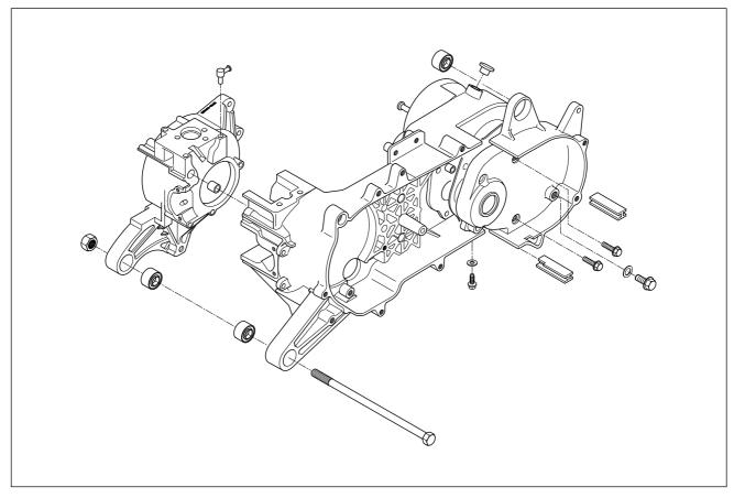
Using two steel tubes of appropriate size, press out the engine mounting bushings on a vise as shown in the illustration.
