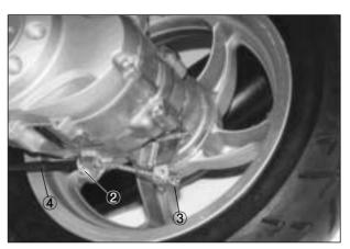
Remove the rear shock absorber mounting lower bolt.
