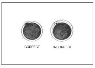
Apply engine oil on the piston pin and install the piston to the conrod.
