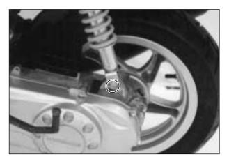
Remove the engine mounting shaft and remove the engine from the frame.
