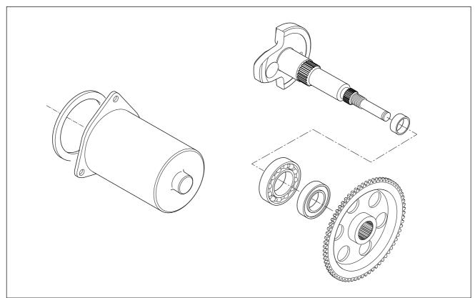
● Install the starter driven gear ② over the left crankshaft end.
