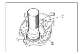
■ Apply SUPER GREASE "A" to the lip of the oil seal ④ and install it to the gear box cover with the special tool.
