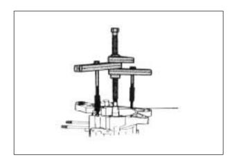
• Remove the crankshaft with the special tool.
