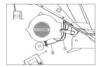
■ Remove the rear brake cable ④ by removing the bolt ①, bolt ② and adjuster nut ③.
