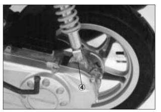
■ Install the magneto lead wire
