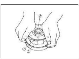
Tighten the clutch shoe nut to the specified torque with the special tool.
