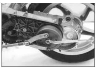
Loosen the clutch shoe nut with the special tool.
