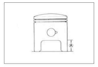
As a result of the above measurement, if the piston-tocylinder clearance exceeds the following limit, overhaul the cylinder and use an oversize piston, or replace both cylinder and piston. The measurement for the bore diameter should be taken in the intake-to-exhaust port direction and at 20mm from the cylinder top surface.
