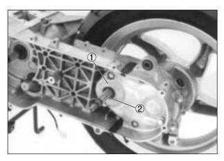
■ Remove the oil seal ① from the gear box cover with the special tool.
