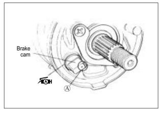
• When installing the cam lever ① to the cam, align the punched mark with the slit of cam lever.
