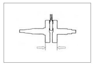
When mounting the crankshaft into the crankcase, it is necessary to pull its left end into the crankcase with the special tool.
