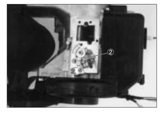
■ Install the reed valve gasket ①, intake pipe gasket ② and intake pipe ④ with reed valve ③ to the crankcase.
