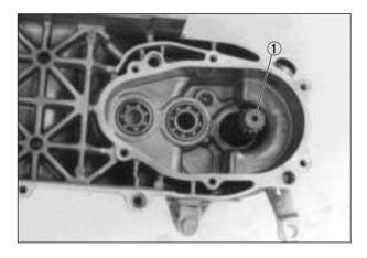
● Apply SUPER GREASE "A" lightly on the rear brake cam pivot part and install it to the crankcase.
