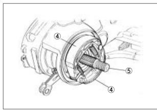
• Remove the bearing retainer 6.
