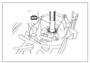
• Remove the oil seal ① with the special tool.
