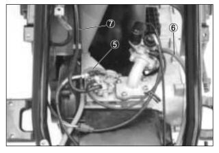
● Disconnect the magneto lead wire ⓐ and starting moter lead wire ⑧.
