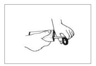
When fitting the oil seal in the crankcase, insert it slowly with the special tools.
