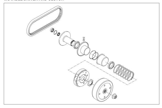
● Install the bearing ② in the fixed driven face ① with the special tool.
