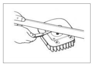
If the largest reading at any portion of the straightedge exceeds the limit, rework the surface by rubbing it against emery paper (of about # 400) laid flat on the surface plate in a lapping manner. The gasketed surface must be smooth and perfectly flat in order to secure a tight joint: a leaky joint can be the cause of reduced power output and increased fuel consumption.
