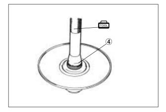
• Install the new oil seals (5), 6) to the movable driven face with the special tool.
