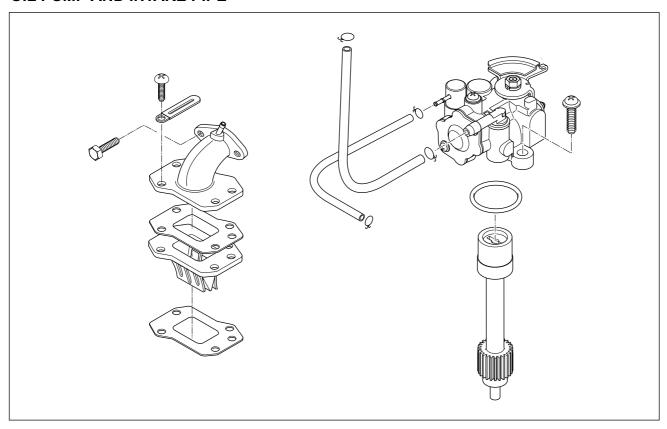
● Apply SUPER GREASE "A" to the oil pump driven gear ① and install it to the crankcase.
