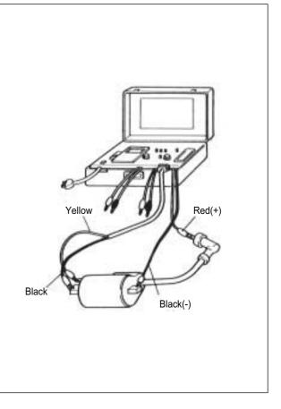
• Check the ignition coil with the pocket tester.
