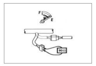
If either one or both indications are abnormal, replace the fuel meter with a new one.
