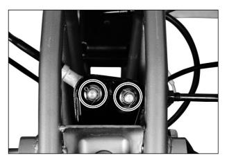
● Separate the tie-rod ends ①, nuts ②, ③ and steering tie-rods ④.
